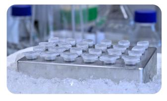
CoolBlock Modules are suggested in applications where your reagents should be cooled or heated uniformly across the wells with ±0.1 °C temperature difference. They can be autoclaved and can be cleaned with alcohol and other disinfectants.
