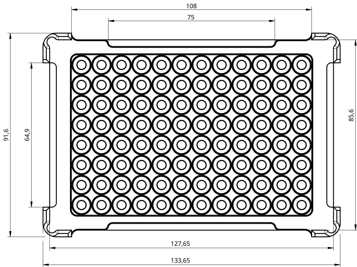
**NOTE:** FOR 96 WELL PLATES, TIP DISTANCE FROM BOTTOM OF THE WELL TO THE BOTTOM OF THE PLATE MIN:28,65mm
